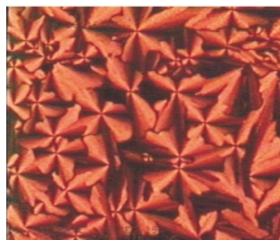
Figure 1. Texture of the liquid-crystalline mesophase of OPV4-PERY-OPV4 between 215 and 310 °C, as observed with polarization microscopy.
